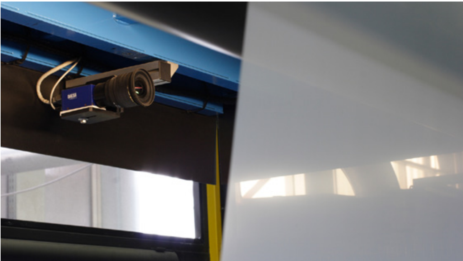
In-line quality control by camera
