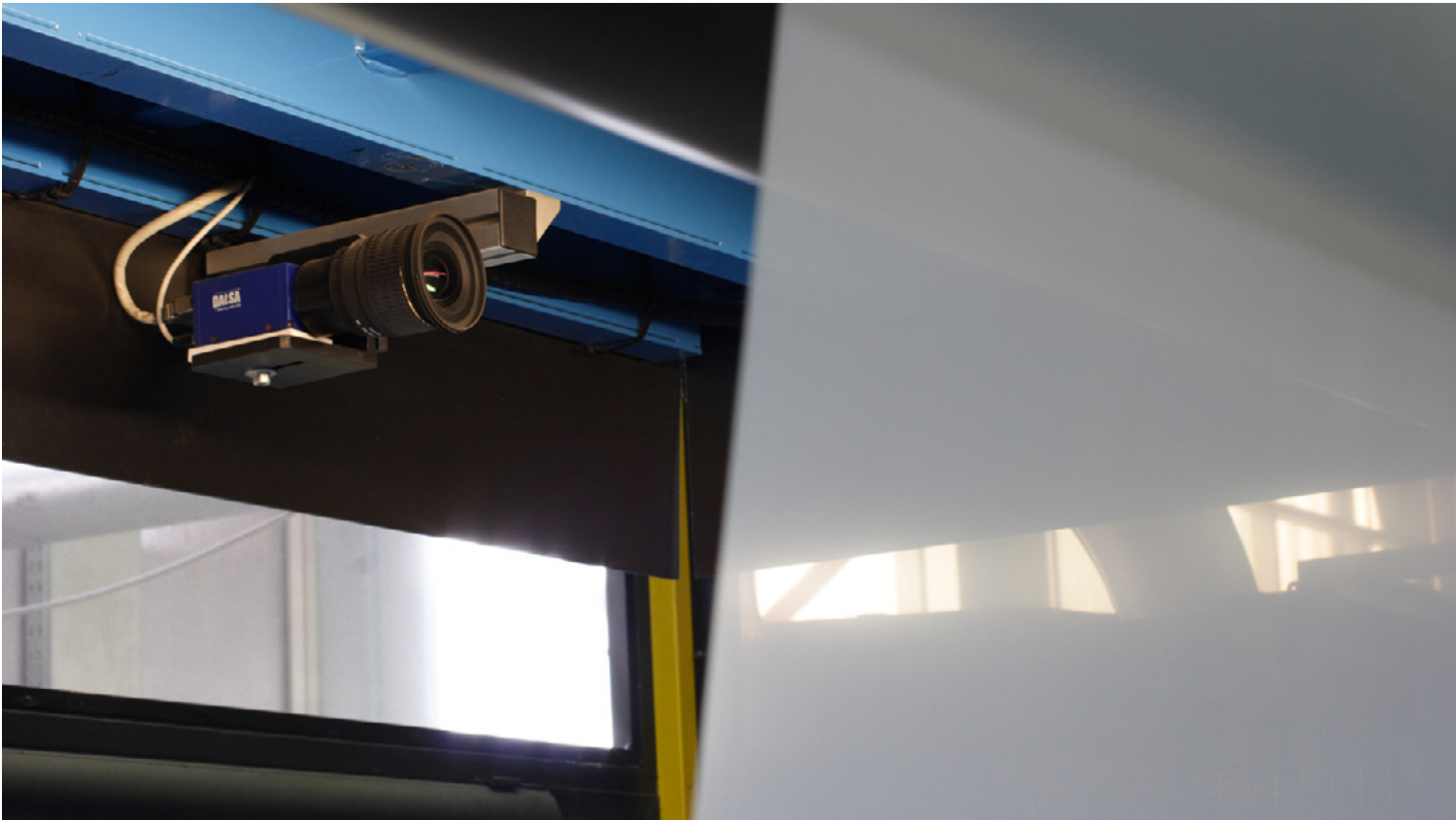
In-line quality control via camera
